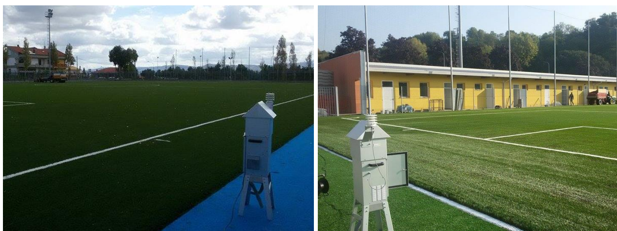
Figure 3- High volume sampler ECHO HI VOL Tecora used for sampling of ambient air.
